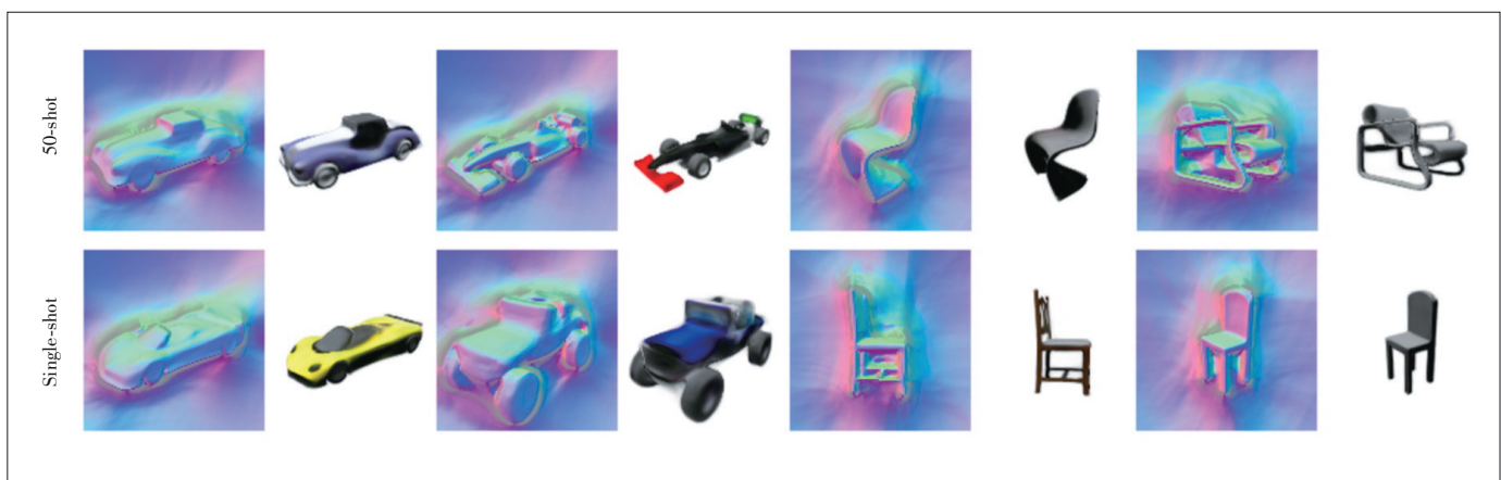
▲ Figure 5. Scene representation networks [17] allow full 3D reconstruction from a single image (bottom row, surface normals and color render) by learning strong priors via a continuous, 3D-structure-aware neural scene representation
