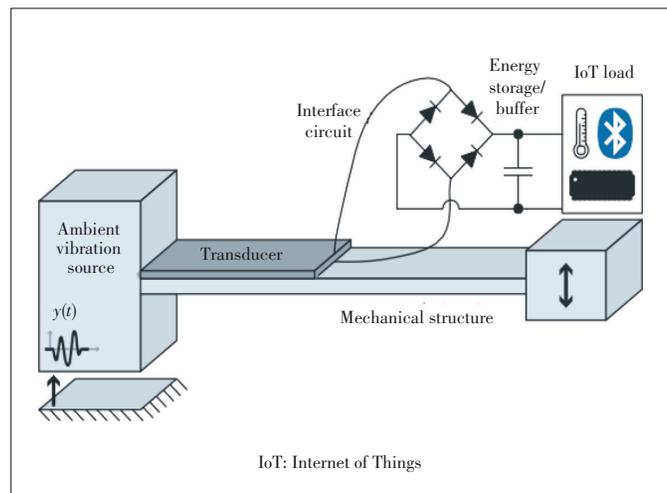
▲ Figure 2. A typical piezoelectric KEH system
