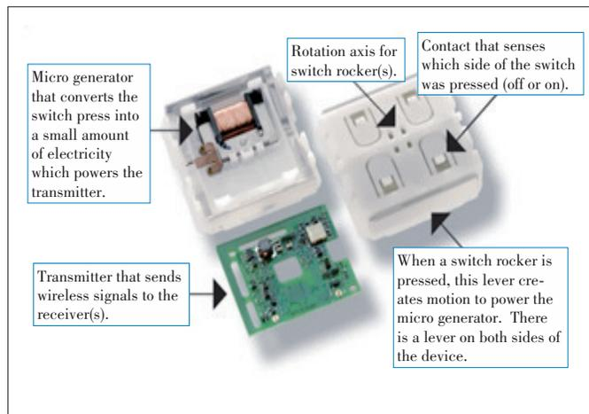
▲ Figure 5. One of the best commercialized KEH-IoT designs, the battery-free wireless light switch developed by EnOcean GmbH<sup>[95]</sup>
