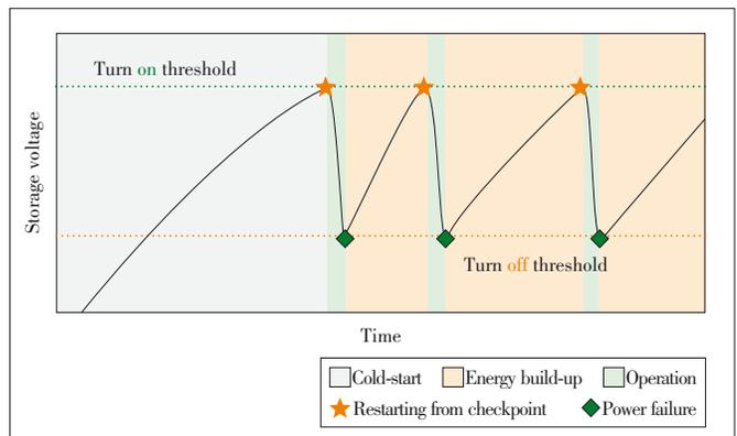
▲ Figure 3. Energy picture during intermittent computing. The energy availability depends on environmental conditions and sometimes also the loading effect. Intermittent execution is a side-effect strategy to cope with this battery-free model, where the blackout periods separating the bursts of execution are unknown
