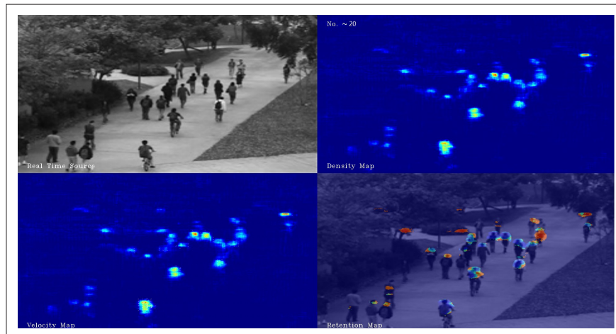
▲ Figure 5. One test video information sampled from the UCSD dataset (from left to right and top to bottom, the four images successively denote real time source, density map, velocity map and retention map respectively).
