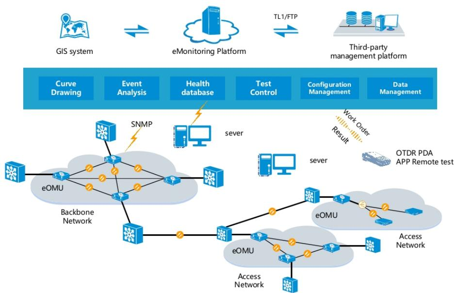
The eServer southbound interface of the eMonitor system is interconnected with the eOMU to collect and analyze optical fiber test data, control tests, obtain and display data, and store and compare health databases. The northbound interface is interconnected with the OSS system to transfer work orders, schedule geographical information, query intelligent optical fiber port information, and implement optical fiber monitoring.
