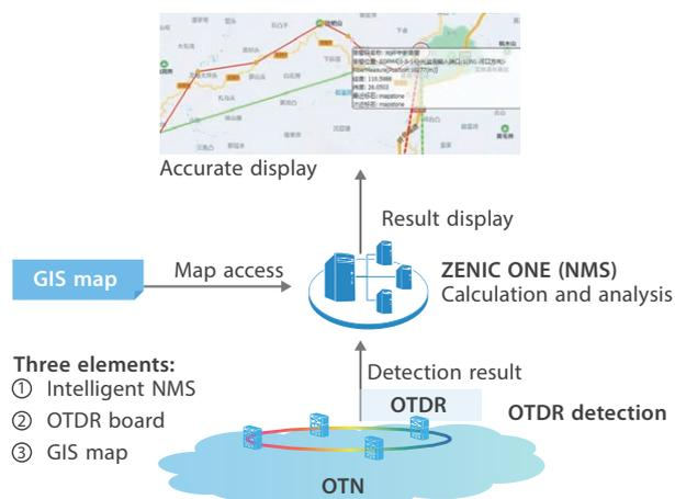
Fig. 1. ZTE's OTDR+GIS-based intelligent fiber fault location system.
