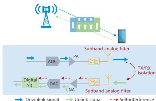
◀ Fig. 1. Design and flexible frame structure of SBFDD RRU.
