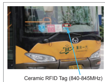
Figure 1. A vehicle with ceramic RFID tag.
