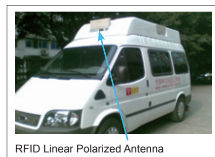
Figure 2. A vehicle with RFID reader and antenna.
