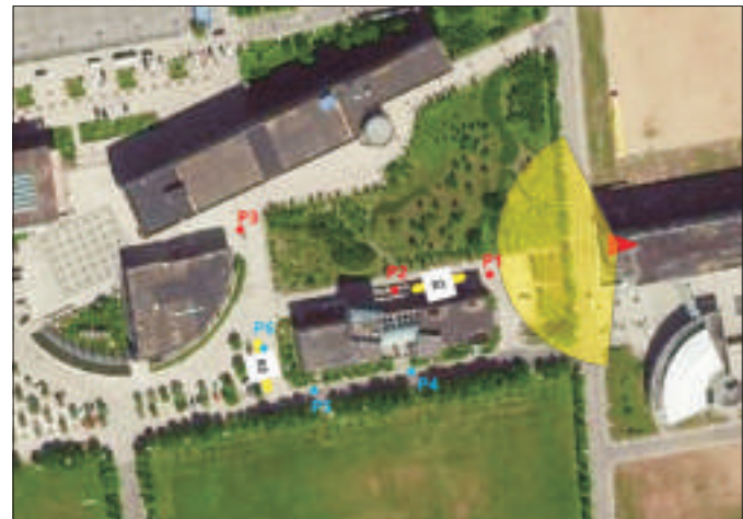
▲ Figure 2. The overview of the measurement area by Baidu Map (The red triangle is the Tx side; two yellow lines, R1 and R2, represent the measurement route in LoS and non-LoS (NLoS) conditions, respectively; and three red points are in LoS conditions while three blue points are in NLoS conditions).
