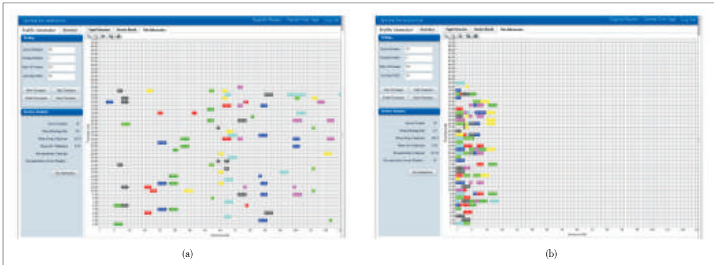
▲ Figure 10. Web view of spectrum defragmentation: (a) before defragmentation; (b) after DfFragmentation.
