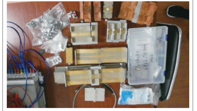
▲ Figure 6. The 6.9 \Omega through reflection line (TRL) measurement fixture
