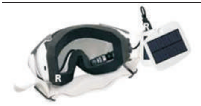
▲ Figure 8. Augmented reality goggles with RFID tag [16].
