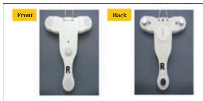
▲ Figure 5. Wearable ECG sensor with RFID tag (indicated by "R") [14].
