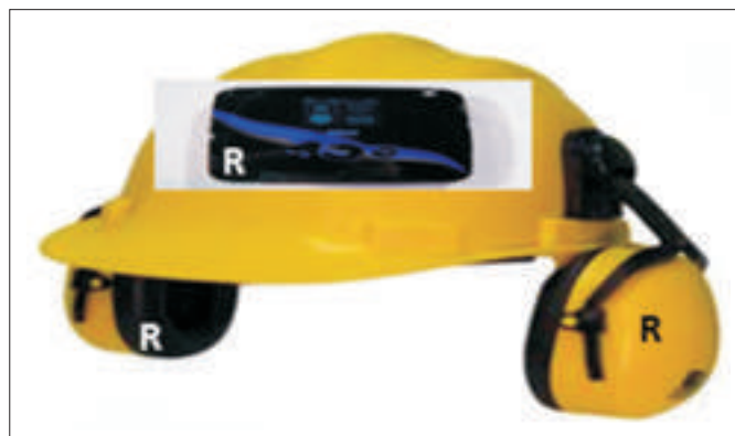
▲ Figure 11. Hat-mountable Verizon JetPack® (by ZTE) with WLAN, GPS, and LTE.
