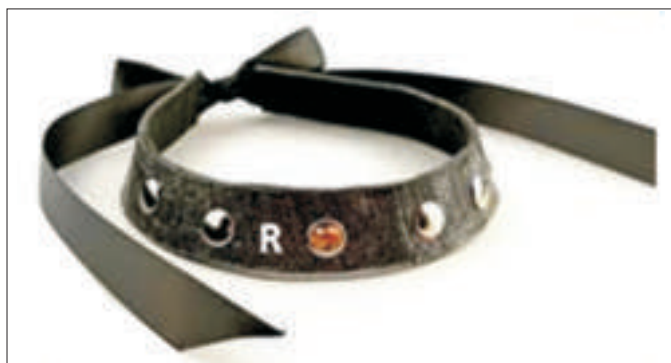
▲ Figure 9. Miniature Bluetooth and Wi-Fi camera embedded into a belt or collar with RFID tag.
