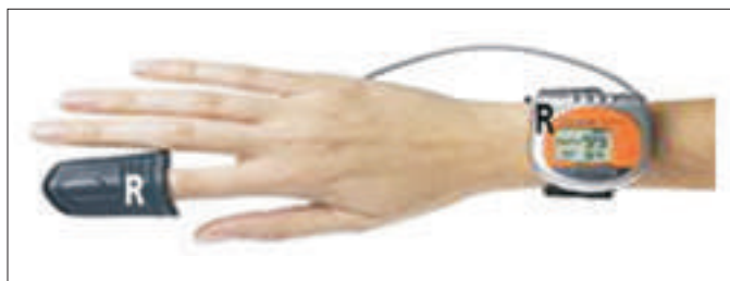
▲ Figure 6. Wearable pulse meter with RFID tag [15].
