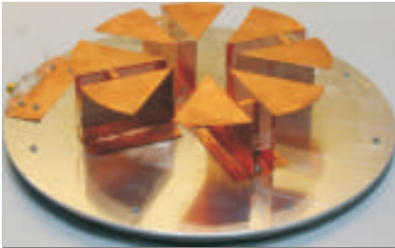
▲ Figure 11. Prototype of a horizontally polarized wideband antenna (in [43] © 2009 IEEE Reprinted with permission).
