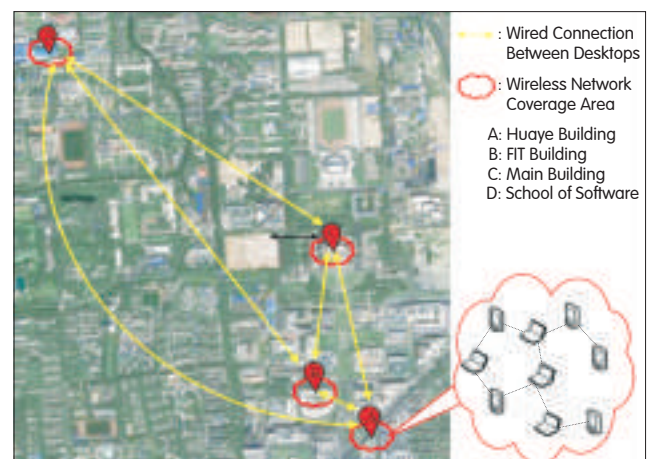
Figure 4. ▶ MoNet experiment network topology with wired network connection. (Here, 106 nodes in 4 different buildings in Tsinghua university are connected using MoNet.)
