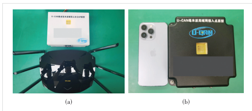
Figure 10. MmWave Wi-Fi modules for: (a) access point and (b) user terminal (Image courtesy of MiSic and Ziwei Tech., etc.)
