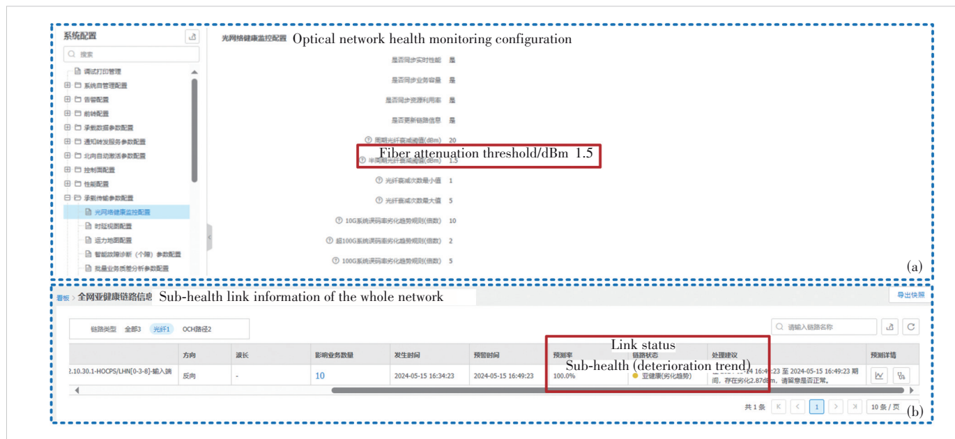
Figure 9. Interfaces of the network management system for (a) optical network health monitoring configuration and (b) sub-health link information
