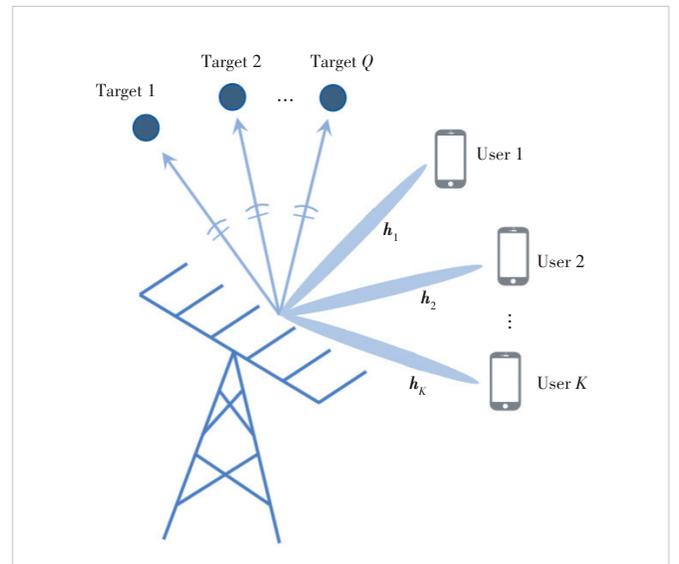
▲ Figure 1. Illustration of the considered dual-functional radar-communication (DFRC) system
