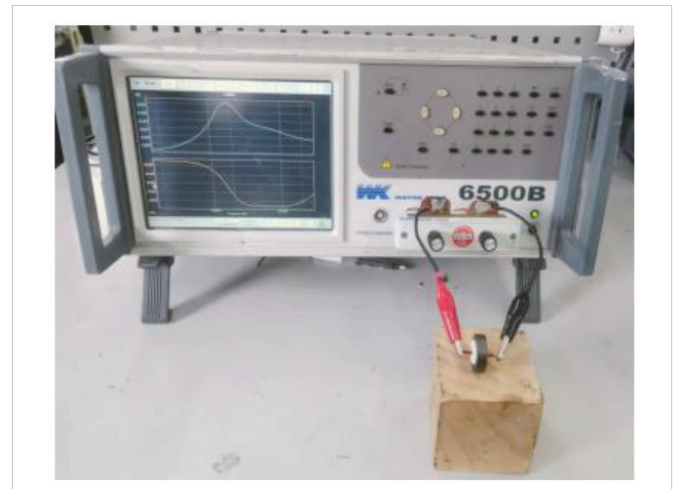
▲ Figure 10. Experimental diagram of the single-turn through-center measurement method
