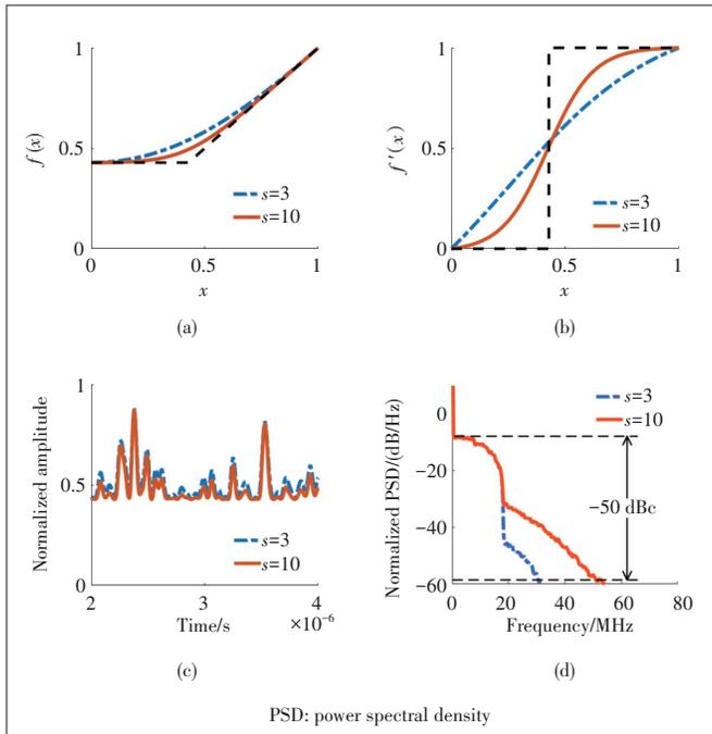
▲ Figure 2. Example of the proposed envelope design: (a) envelope design; (b) derivative of the S function for  $s=3$  and  $s=10$ ; (c) time domain waveforms; (d) normalized power spectral density of the S envelope
