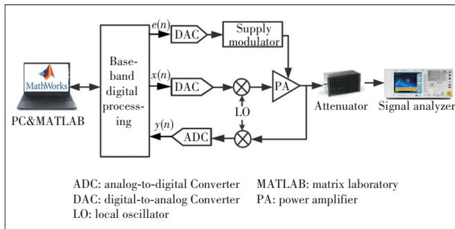
▲ **Figure 3.** Test bench setup
