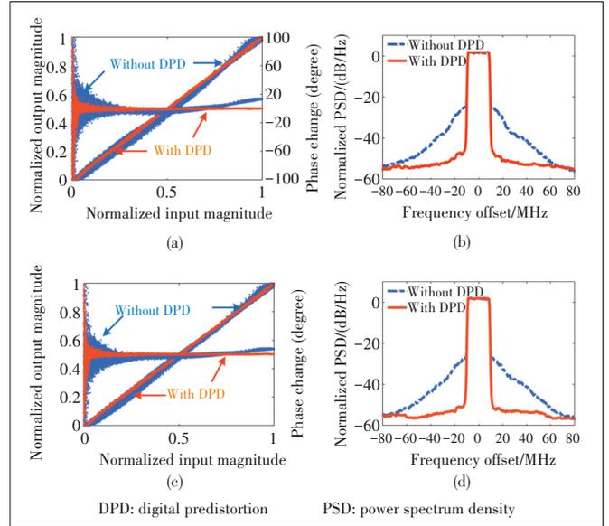
▲ **Figure 5.** Comparison experiment: (a) amplitude-modulation to amplitude-modulation (AM/AM) and amplitude-modulation to phase-modulation (AM/PM) curves; (b) normalized PSD without and with DPD under S10 function; (c) AM/AM and AM/PM curves; (d) normalized PSD without and with DPD under Wilson function
