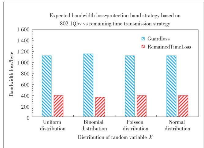
▲ Figure 6. Comparison of the expected bandwidth loss between the remaining time transmission strategy and the guard band strategy of 802.1Qbv
