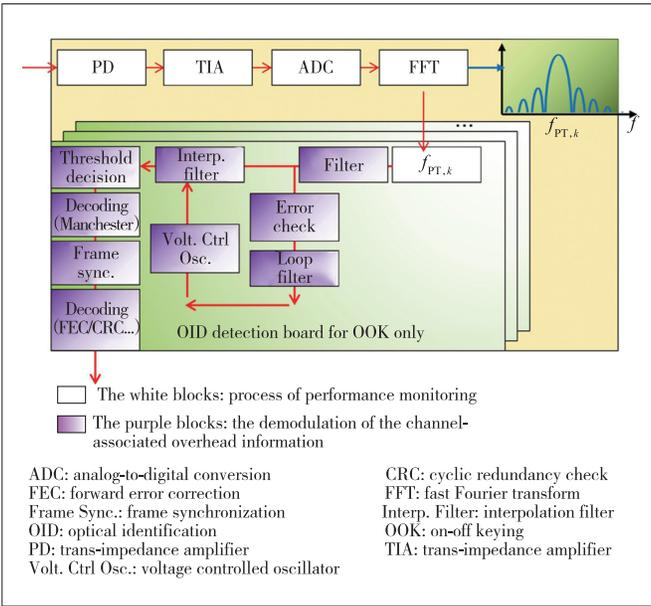
▲ Figure 2. OID detection process, taking OOK modulation as an example
