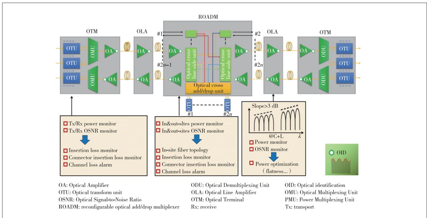
▲ Figure 4. Schematic diagram of optical channel layer (OCh) performance monitoring and management based on OID tool
