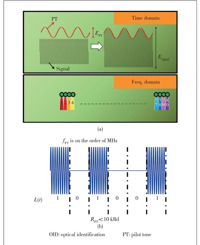
▲ Figure 1. Schematic diagram of (a) OID loading and (b) channel-associated overhead data
