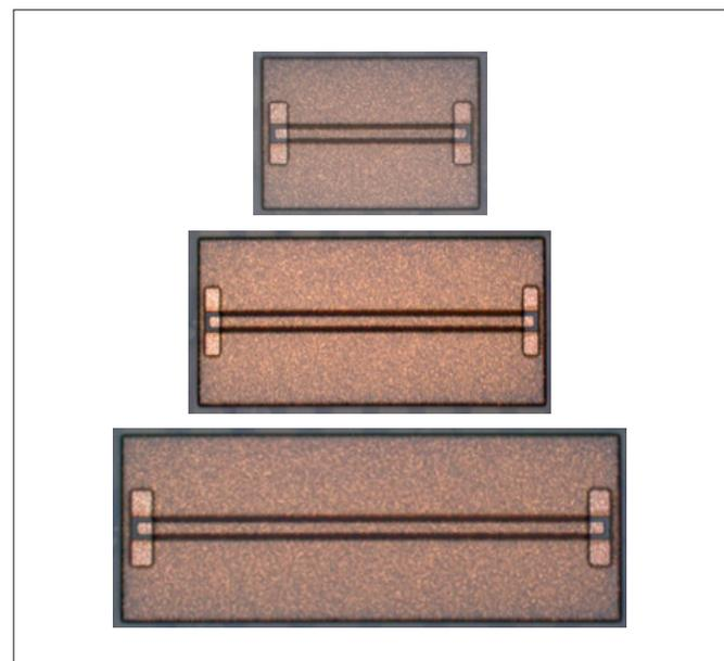
▲ **Figure 2.** Coplanar waveguide (CPW) with 3 different lengths.
