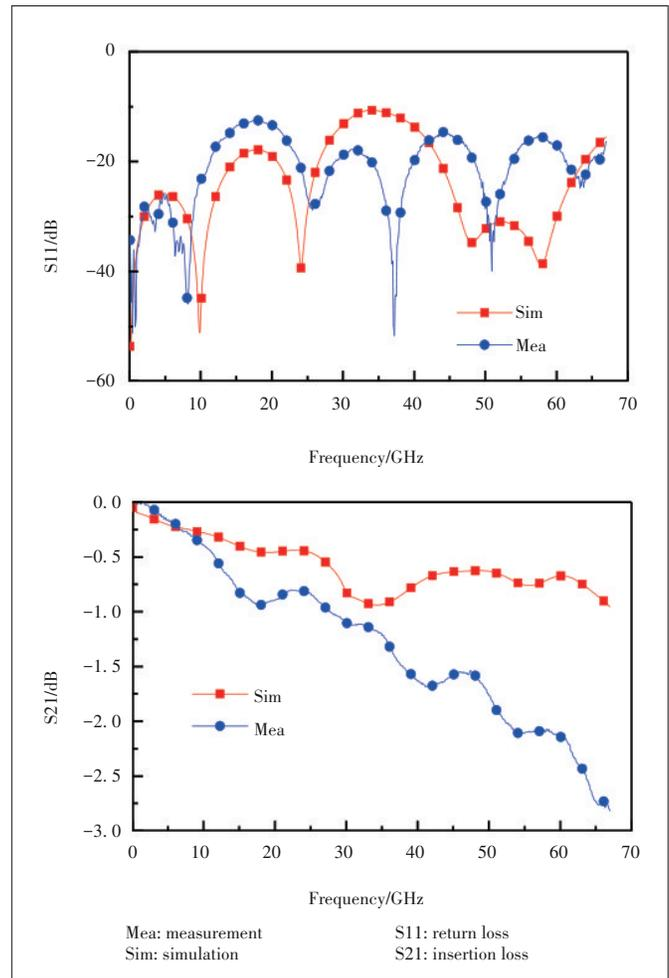
▲ Figure 6. Comparison between test and simulation results of 3D stacking coplanar waveguide (CPW).
