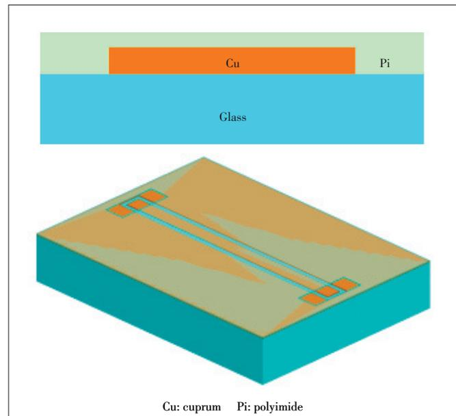
▲ **Figure 1.** Structure of coplanar waveguide (CPW).
