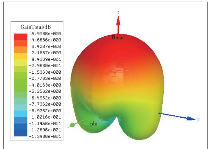
▲ Figure 11. Radiation pattern of antenna.
