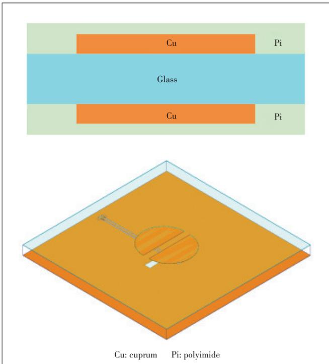
▲ Figure 7. Antenna structure and geometry.
