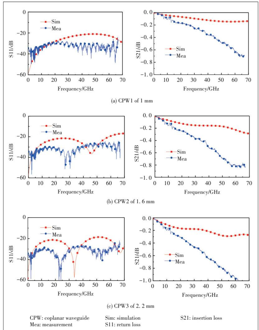
▲ **Figure 3.** Comparison of test and simulation results of CPW.
