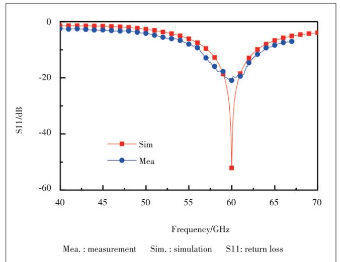
▲ Figure 10. Reflection coefficient of antenna.
